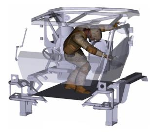
Could a fully equipped Warfighter exit this design in an emergency? Don't guess. Let Santos enable your engineers to conduct assessments like this well in advance of prototyping.
