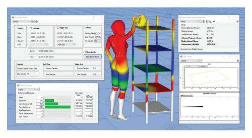
SantosHuman Inc.'s unique physics-based digital human modeling software has been used by manufacturers of automobiles, heavy equipment and consumer goods. In this case, the company performed complex simulations to shape the optimal laundry bottle. CREDIT SANTOSHUMAN INC.
